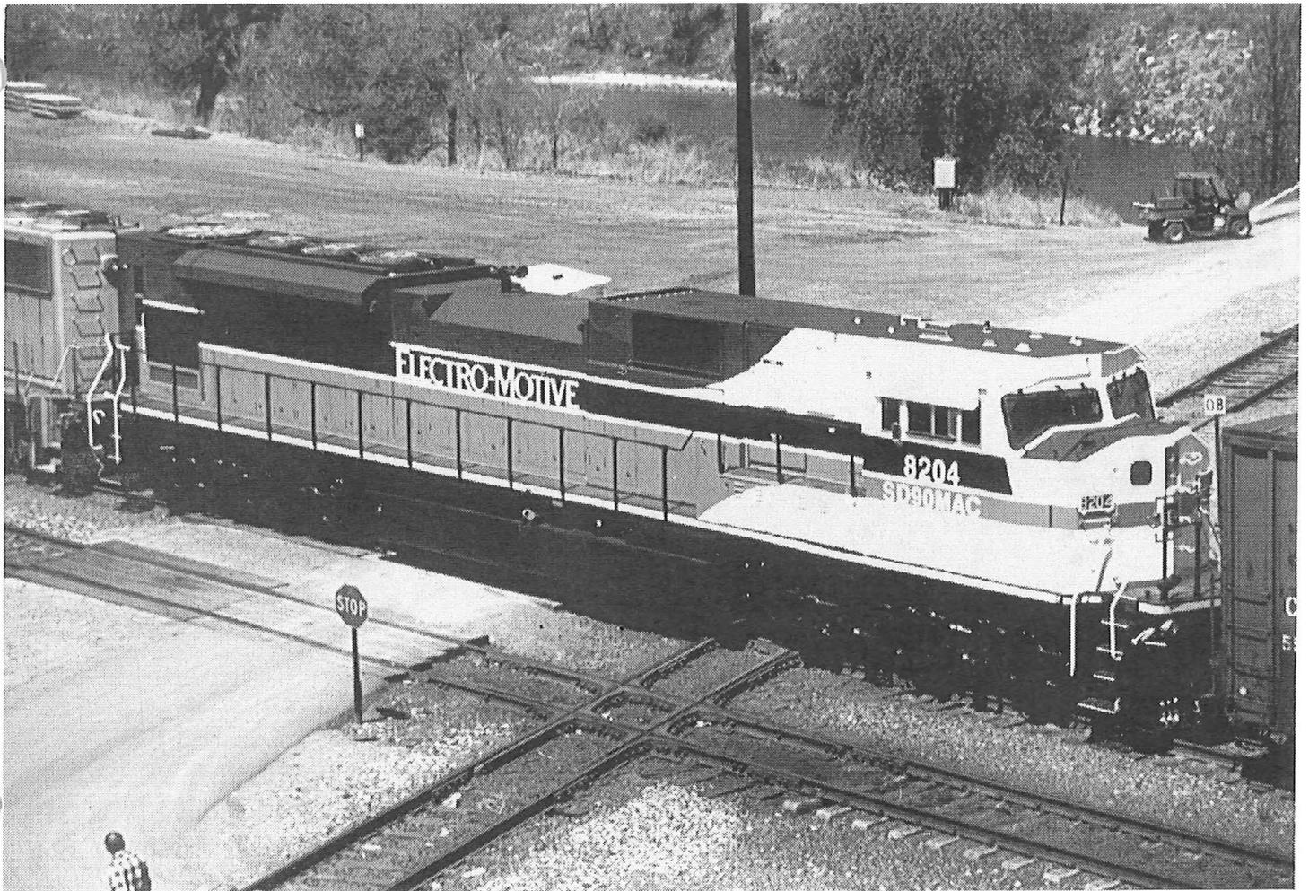
*EMD SD90MAC #8204 was at the BNSF 23rd Street crossing on the BNSF train H-DENFTWI-09 enroute to the Transportation Test Center in Pueblo, CO, on May 9th, 1997. The unit sports EMD's 75th Anniversary paint scheme. This is EMD's newest 6,000 horsepower, AC-powered demonstration model. (Chip Sherman Photograph)*
