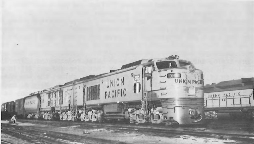
*Do you remember these big beauties? Dick Kindig photographed the Union Pacific's gas-turbine electric #1 at Cheyenne, on October 13, 1962. Delivered to the UP in 1958, these 8,500 hp "Big Blows" were two units, permanently coupled and equipped with auxilliary heavy oil tender.*
