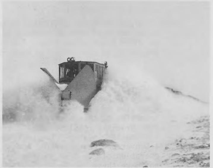
*Union Pacific double track wedge plow 900020, and four diesel units, pause at Centennial, Wyoming (left), while opening the Coalmont Branch on January 9, 1979. The next day, UP Jordan Spreader 903031 (right), on the point of an empty coal train, busts a drift just east of Centennial, in typical winter Coalmont Branch action. (Jim Ehemberger Photos)*
